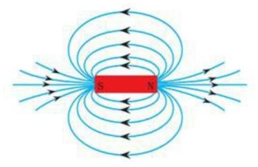
**Ans.** The space or region where field is same everywhere is known as Uniform magnetic field. The magnetic field which is unequal in magnitude and direction at every point in the space is called non- uniform magnetic field.
