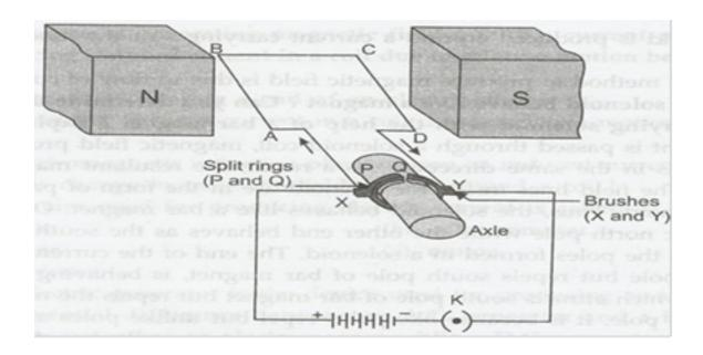
**Principle:** A current-carrying conductor, when placed in a magnetic field, experiences a force. If the direction of magnetic field and that of current are mutually perpendicular then force acting on the conductor will be perpendicular to both and will be the given by Fleming's left-hand rule. Due to this force the conductor begins to move, if it is free to rotate.
