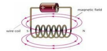
**Ans.** A solenoid is a coil of many turns of insulated copper wire closely wound in the shape of a ring.
