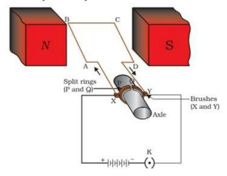
3. Draw a labelled diagram of an electric motor. Explain its principle and working. What is the function of split ring in an electric motor?
